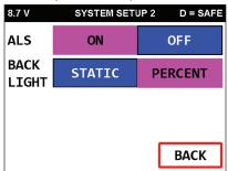
**ALS** – Turns the Automatic Light Sensor **ON** or **OFF**. When this function is on the Backlight button is disabled.
