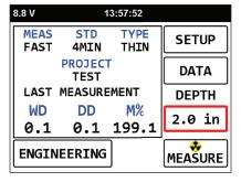
Press the value under **DEPTH** 2.0 in button on the screen to select the desired thickness for the material being measured.
