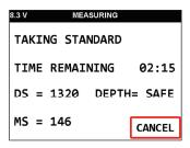
After the standard count has completed, the display will show the new standard with % error derived from the last four standard counts. If the errors are outside these limits refer to the important notice above. If the above conditions are normal, then press **RETAIN THE NEW STD** and take a new standard as above in 3.2. Repeat taking new standard for a maximum of four times to reduce to within the limits.
