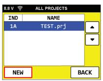
Note: The "A" next to the number in the index column indicates the project is active. **TEST** is the current active project as seen below.
