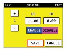
Now the Field Calibration is saved and enabled. Every measurement taken in Backscatter will now be reduced by 1 percent.
