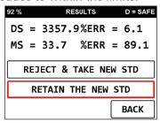
If the error is below 1% and 2% for DS & MS respectively then the display will show just the DS and MS counts as seen below:
