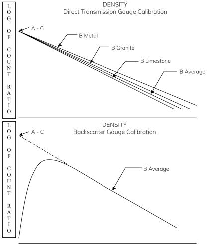
Fortunately the most common materials in the surface layers are oxygen, silicon and calcium in the form of oxides or carbonates. If this were not the case, Gamma Density Gauges would not be practical for use. These materials all have a u/p between 0.0805 and 0.0809. Large amounts of hydrogen in surface water do require an adjustment in the measured density.
