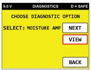
It will prompt you to place the gauge on the reference block, which is important to take moisture readings.
