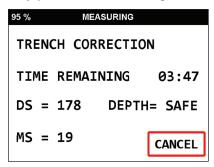
When the count is complete both the Density and Moisture Correction Factor will appear on the display, which is the difference between the Moisture Standard Count outside of the trench and the same standard inside the trench.
