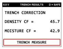
Press **TRENCH MEASURE** to take the measurement in the trench. After the measurement is completed, the gauge will display the results based off the trench correction factors.
