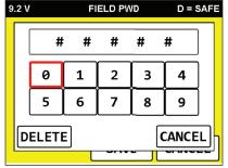
In this example we will set a Field Calibration for BS to -1.0% in position 1. Press the value box under BS and a popup keypad will appear.
