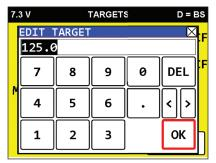
Press **OK** on the screen when you have entered the desired target value. Press **BACK** on the next screen to save any changes.
