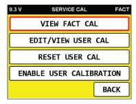
Here you can view the factory calibration constants for each depth. Press the + or – key to advance to the desired depth as seen below:
