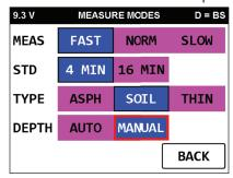
When the gauge is in Manual Mode the Main Screen will now show an outlined button around the **DEPTH** position as seen below:
