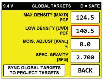
Press **LOW DENSITY** [LWD] value on the screen and the **EDIT TARGET** keypad will pop up as shown below:
