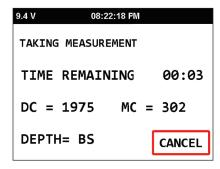
After the **TIME REMAINING** counter has elapsed. The Wet Density (WD) and Percent Marshall (%MA) will appear on the display. Since the moisture channel is measuring Hydrogen, the displayed results will approximate the Asphalt Content (AC) of the mix. The depth of measurement will be 100mm (4 inches) or even more depending on the actual asphalt content.
