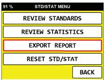
Pressing **RESET STD/STAT** will clear the registers of the current standards and reload the standards from the factory calibration.
