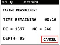
After the **TIME REMAINING** counter has elapsed. The Dry Density (DD), Wet Density (WD), Percent Moisture (%M), Wet Density (WD), Moisture Content (M), and Percent Proctor (%PR) will appear on the display.
