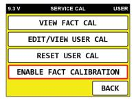
Pressing RESET USER CAL will reset the user calibration to match the
