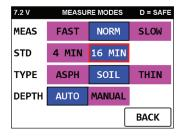
Press 16 MIN to change the **STANDARD** mode to **STATISTICAL** mode and press the **STD/STAT** button to jump to the **NEW STANDARD** menu as shown below:
