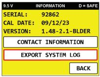
A system log will be created on the **USB** drive in a (.txt) format.
