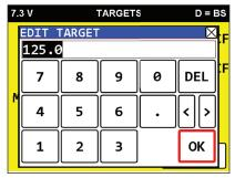
Press **OK** on the screen when you have entered the desired target value. Press the **BACK** button on the next screen to save any changes.
