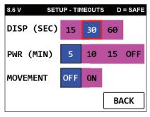
**DISP** (SEC) – This will set the timeout in seconds as to when the gauge will go into sleep mode. Pressing any key or touching the display will wake it back up.
