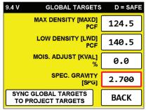
Press **SPEC. GRAVITY** [SPG] value on the screen and the **EDIT TARGET** keypad will pop up as shown below:
