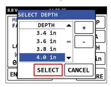
Using the + or - Keys on the screen select the desired depth and press Select to accept.
