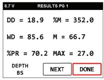
The gauge will not stay in Trech Correction mode after the test is done. Every trench measurement will need to have an individual the Trech Correction prior to taking a measurement.
