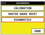
From the Diagnostics menu you can view Moisture, Density, High Voltage and Battery Voltages.
