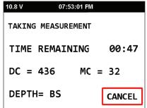
**NOTE:** If the gauge is in low power mode (Power on Screen off) when pressing the **MEASURE** key, a warm up period of about 10 seconds will elapse to bring the electronics and detector tube signals up to a stable level before measurement can begin.
