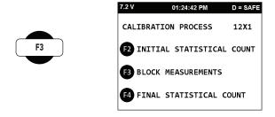
Press **F3** to move the highlighted field to the correct calibration block. Press **F4** to enter the **NEXT** screen.
