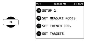
From the **SET TARGETS** menu, Press **F2** to edit the **KVAL%** with the "+" highlighted as shown.
