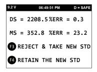
Errors within 1% for density and 2% for moisture counts are expectable. If the errors are outside these limits refer to **Important notice** above. If the above conditions are normal, then press (**F4 RETAIN AND TAKE NEW STANDARD**) and take a new standard as above in 3.2.
