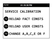
Press **F2** to Reload the **FACTORY** Constants. Press **F3** to Reload the **USER** Constants. Press **F4** to **CHANGE** the **A, B, C, E** and **F** parameters.
