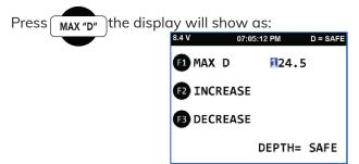
The current value of the maximum density target will be displayed and the left most field will be highlighted. Press **F1** to cycle the highlighted cursor to the right by one field at a time. Pressing **F2** will **INCREASE** the value that is highlighted, while pressing **F3** will **DECREASE** the highlighted value.
