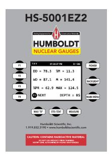
Control panel Image is shown indicating the positions of the display and keys. The keys are grouped across the bottom for easy access and the display labeled for clarity.
