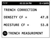
Remove the Gauge from the Reference Standard, place the Gauge on the site to be tested (always use direction transmission in a trench) and take a normal soil measurement. The measurement result has been adjusted to compensate for the water in the wall of the trench.
