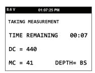
**NOTE:** If the gauge is in low power mode (Power on Screen off) when pressing the **MEASURE** key, a warm up period of about 10 seconds will elapse to bring the electronics and detector tube signals up to a stable level before measurement can begin.
