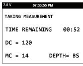
After the **TIME REMAINING** counter has elapsed. The Dry Density (**DD**), Wet Density (**WD**), Percent Moisture (**%M**), Wet Density (**WD**), Moisture Content (**M**), and Percent Proctor (**%PR**) will appear on the display.
