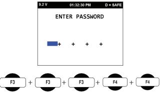
To enter the password, press the following function keys in sequence, F3+F3+F3+F4+F4.
