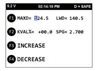
Press F1 to move the highlighted field for MAXD and LWD. Press F2 to move the highlighted field for KVAL% and SPG. Press F3 to INCREASE the value in the highlighted field. Press F4 to DECREASE the value in the highlighted field.
