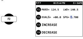
Pressing **F2** will shift the highlighted cursor one field to the right to allow the user to edit the highlighted value. Press **F3** to **INCREASE** the highlighted value, otherwise press **F4** to **DECREASE** the value.
