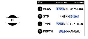
Press **F1** to advance the field to the right (**FAST / NORM / SLOW**) until the desired measurement time selection is highlighted.
