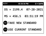
**DS** and **MS** are the values of last density and moisture standards taken at the date **MM/DD/YY** and time **MM:HH:SS**. If you wish to take another standard press **F3**, otherwise press **F4** to use the current standard and go back to the main menu.
