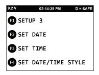
Press **F1** to change the highlighted **DATE** format. Press **F2** to change the highlighted **TIME** format. Press **F4** to **SAVE** the desired formats.
