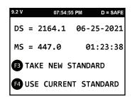
Where **DS** and **MS** are the values of the last density and moisture standard take on date **MM/DD/YYYY** and time **HH:MM:SS**. If another standard is required press **F3**, otherwise press **F4** to use the current standard and go back to the main menu.
