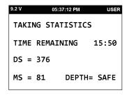
After the **STAT** test is complete, and there was no error in DS & MS the display will show:
