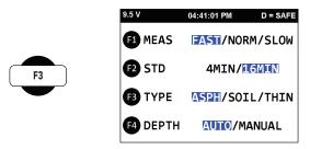
Press **F3** to advance the field to the right (**ASPH / SOIL / THIN**) until the desired measurement type selection is highlighted.
