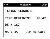
After the standard count completion and there are no errors in the standard counts, the display will show:
