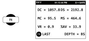
The Density Counts (**DC**), Density Standard (**DS**), Moisture Counts (**MC**), and Moisture Standard (**MS**) will indicate the counts used to determine the computed data. The Void Ratio (**VR**) and Percent Air Voids (**%AV**) are calculated along with the **DEPTH** at which the measurement was taken.
