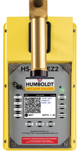
After each test, a QR code is presented on the EZ-2 Screen. Scanning this code transfers the data to the phone app. The NX transfers wirelessly. Both allow you to share the data with others via email, text message or a cloud-sharing platform.
