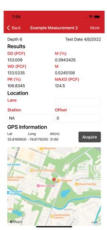
Typical informaton displayed on the phone app includes: time of test, dry density, moisture percent, wet density, moisture, percent of proctor, maximum density, as well as the location, the GPS informaton and a map illustrating the test location.
